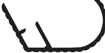
Front Gutter (C)
