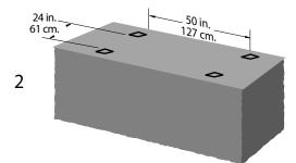
(Measurements shown are inside to inside of posts)
